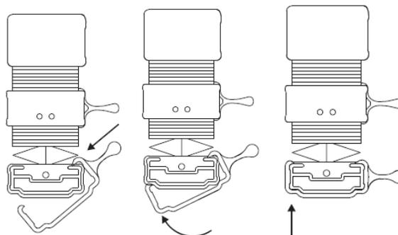
For shades  $W \leq 38''$ , single cordless handles should be operated from the center of midrail and bottomrail.
