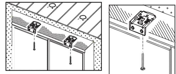
Make sure both brackets are aligned. "L" shape opening should be facing down, with longer side against top of the window opening.
